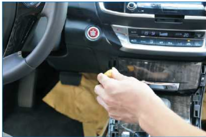
2、拧开储物盒左右固定螺丝并将储物盒拆下。 2. unscrew the left and right screw and use fry tool to remove the plastic board
