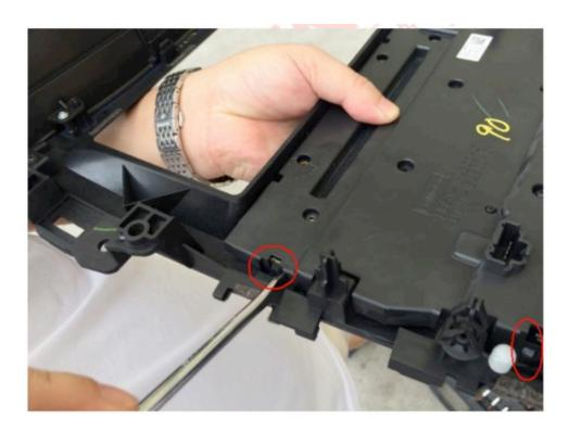
3) Disconnect the three cables circled in green on the air conditioning control board and remove the screws circled in red
