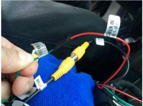
12, remove the board inside OEM USB / AUX box, and replace with USB board supplied with the new unit, then connect USB adapter cable, the other end of the adapter cable goes to a USB port of the new unit, connect the connectors(power harness, video/camera harness,
