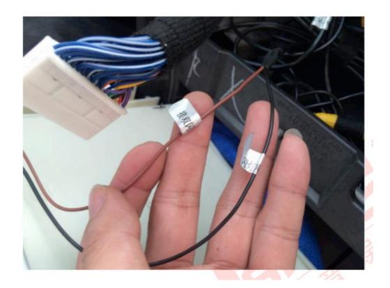
15, put the air conditioning control panel prepared in step 8 into the car storage box and connect the connector at the back, then tap the black and brown hazard light extension wires into the the lines of the connector indicated below
