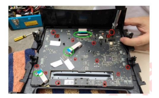
4) Remove the screws that secure the frames and then remove the upper and lower frames
