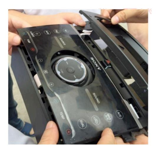
5) Pull out the air conditioning control knob and remove the chrome ring
