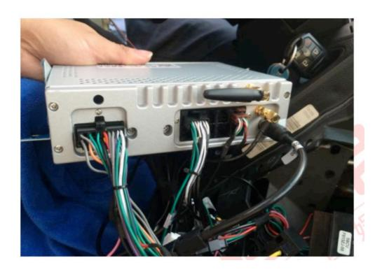
13, Secure mounting brackets, and then secure the brain of the new unit to the  $\operatorname{\mathsf{car}}$
