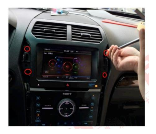
3. Remove the OEM face panel, and remove the connectors at the back  $% \left( 1\right) =\left( 1\right) \left( 1\right)$
